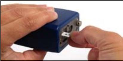
4. Make sure that the flow calibration kit is connected to the AE51.
