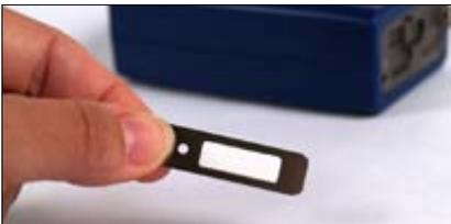
Metal side of filter strip faces the bottom.
