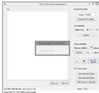
13. Repeat steps 9-12 for all flow setpoints in the dropdown menu in the Manual calibration section of the software.
