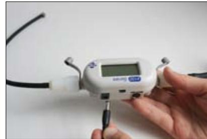
2. Connect the mini-DIN end of the 2-part flowmeter computer cable to the flowmeter. Connect the USB end of this cable to the computer with the software installed.
