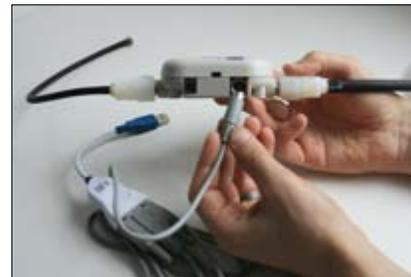
3. Screw the 10-32 threaded elbow fitting connected to the outlet port of the flowmeter to the inlet port of the microAeth AE51 (10-32 threaded elbow fitting connected to 1/8" tube WITHOUT the In-line 60mm round ULPA Filter). On the rear panel, opposite of the flowmeter LCD screen, there is an arrow denoting the direction of air flow through the flowmeter. **Be careful to ensure that the elbow fitting o-ring face seal seats properly against the AE51.**
