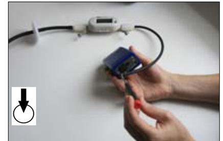
4. Connect the USB cable to the microAeth AE51 and your computer using the USB cable that was provided with the AE51.
