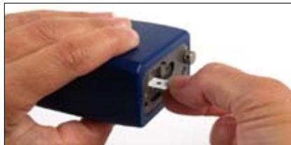
7. Install a new filter strip by pressing and holding the release button and then inserting the new filter strip into the sample chamber opening.
