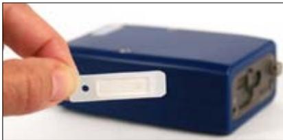
White sample deposit side of filter strip faces the top.
